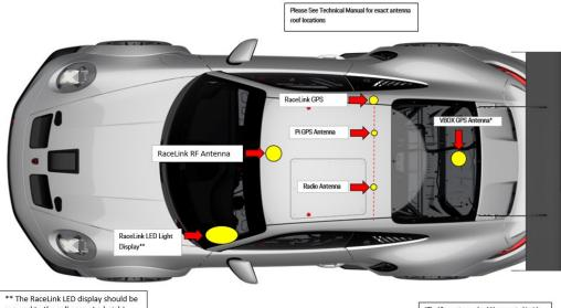
\*\* The RaceLink LED display should be secured to the roll cage at a height equal to the marked eye level mark required for the containment nets. (See Appendix 2)
