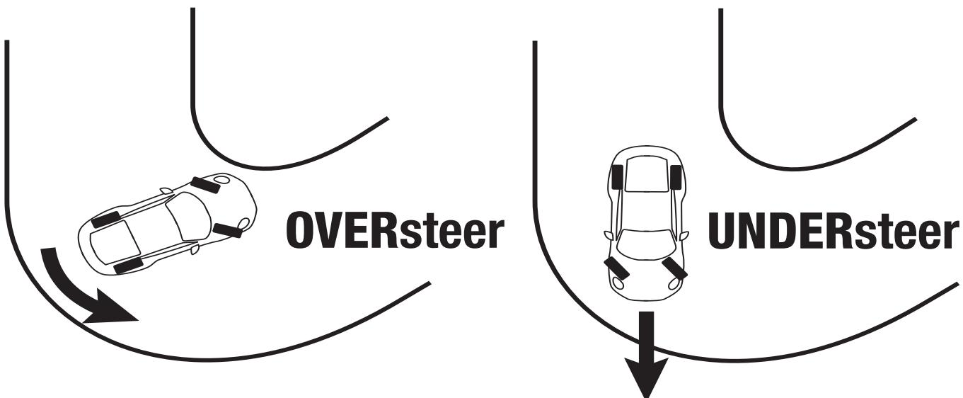
**OVERSTEER:** A car oversteers, or is “loose,” when, as you turn the steering wheel, the car wants to turn more than what your input calls for. The rear end of the car starts to slide out due to loss of traction.
